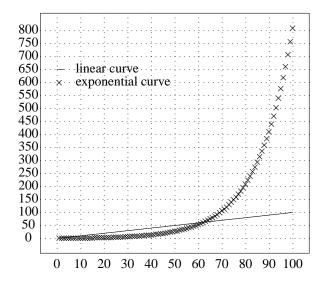
Produced by GROWTHFACTOR=0.07 grid bot dotted from 0 to 100 by 10 grid left dotted from 0 to 800 by 50 frame ht 2.5 wid 2.8 define expo { \$1+\$1\*GROWTHFACTOR } value = 1 draw LINEAR solid for i from 1 to 100 by 1 do { next LINEAR at i, i times at i, value value = expo(value) 111egend=650 12legend=600 line from 0,111egend to 3,111egend times at 1,121egend "linear curve" ljust at 8,111egend "exponential curve" ljust at 8,121egend label top "Exponential curves: growth over time (7%)" up -.2
